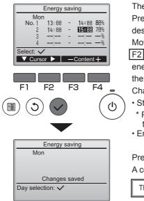
The pattern setting screen will appear. Press the F1 button to move the cursor to the desired pattern number.
